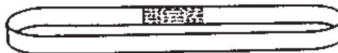
Endless sling, may be fully open or sewn full length with stitched soft eyes
