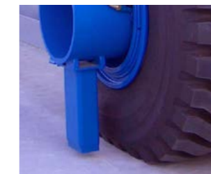
Drop stops prevent damage in case of tyre deflation
