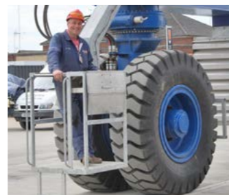
Low mounted drivers stand constructed from 316 stainless and galvanised steel
