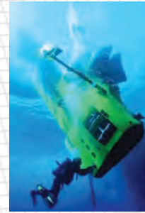
Divers re-rigging Enclosed Flotation Bags 2,000 lbs. on James Cameron's Deepsea Challenger.
