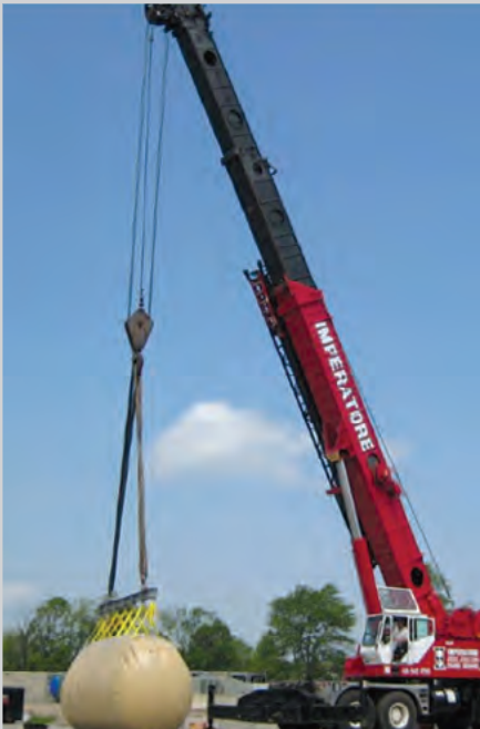
Product proof load testing of Salvage Pontoon 70,000 lbs.
