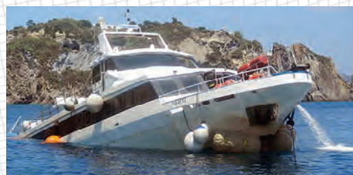
Yacht salvage using Salvage Pontoons 2,000 lbs. and Salvage Pontoons 20,000 lbs. Photo credit: Vessel Assist - San Diego.
