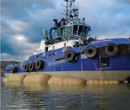
SP-70000's and SP-40000's used to reduce the draft of a newly constructed tugboat during launch. Photo Credit: Ocean, Quebec, Canada.
