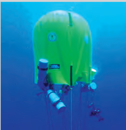
Custom inflatable underwater decompression habitat used by Michael Lombardi with National Geographic
