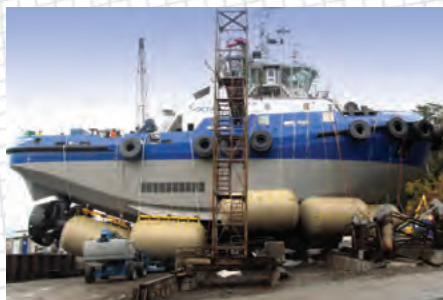
Draft reduction for newly constructed tugboat launching using Salvage Pontoons 40,000 lbs. and Salvage Pontoons 70,000 lbs.
