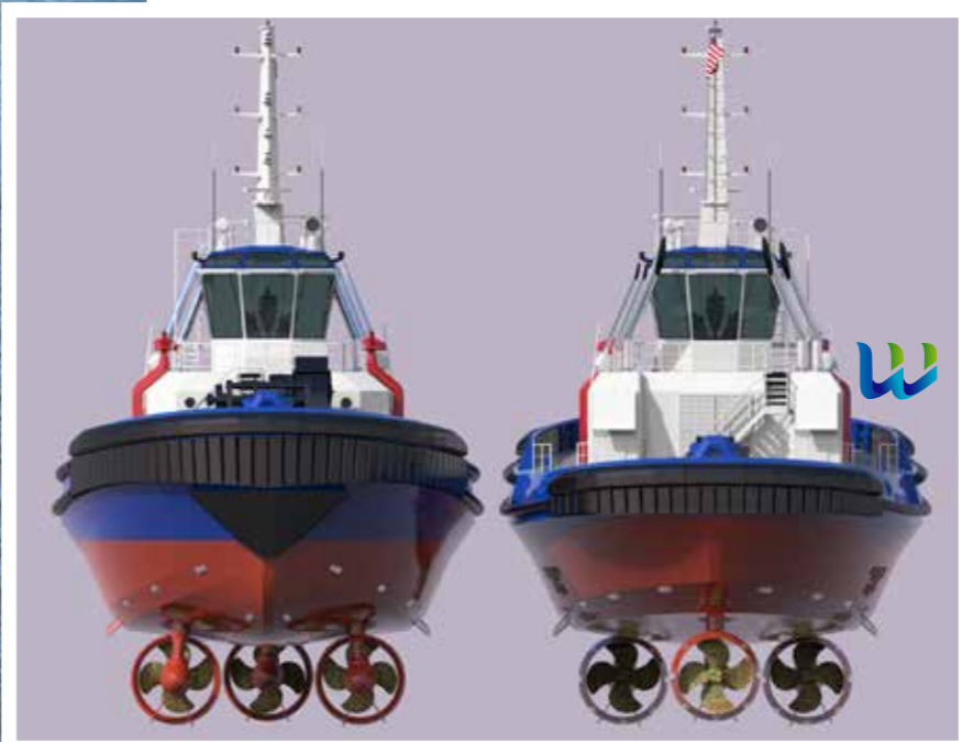
Tug Fender layout with Modular Cylindrical and W-Fender replacement sections.
