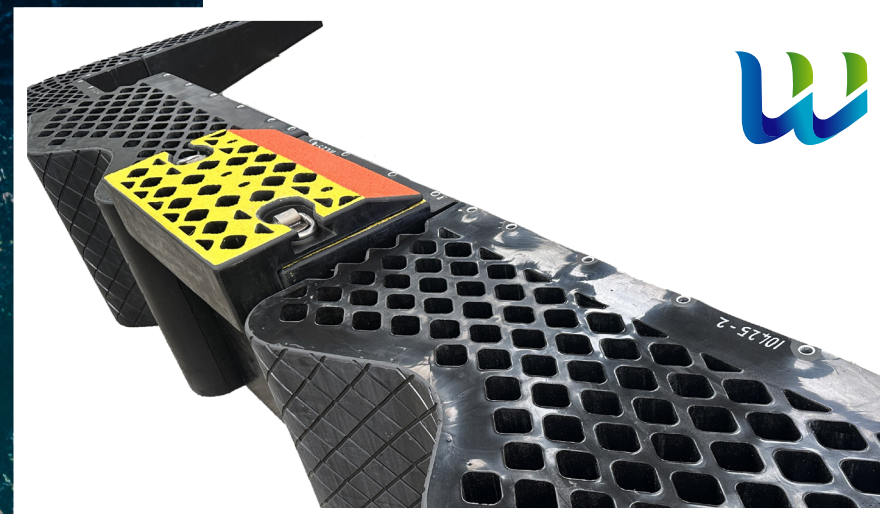
CREW TRANSFER VESSEL BOW FENDER ARRANGEMENT with impact fenders and step unit.
