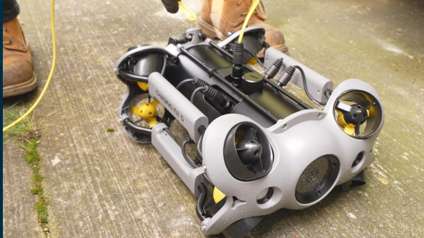
Fig1 Connect the drone to the tethering cable
